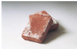
3-Thick Half Brick Flat(半マス倍厚平)
